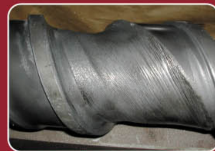
105 mm feed screw before coating. After 3 months of 40% glass filled Nylon
