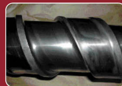
The same screw with carbide coating after 10 months in the same process
